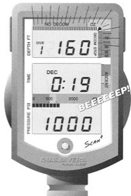
Figure 24 Delayed Violation - Deco stop greater than 40 feet
